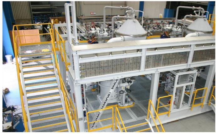
GEA has delivered two centrifuges for monoethylene glycol (MEG) purification at BP's West Nile Delta offshore n field in Egypt. Photo credit (GEA)
